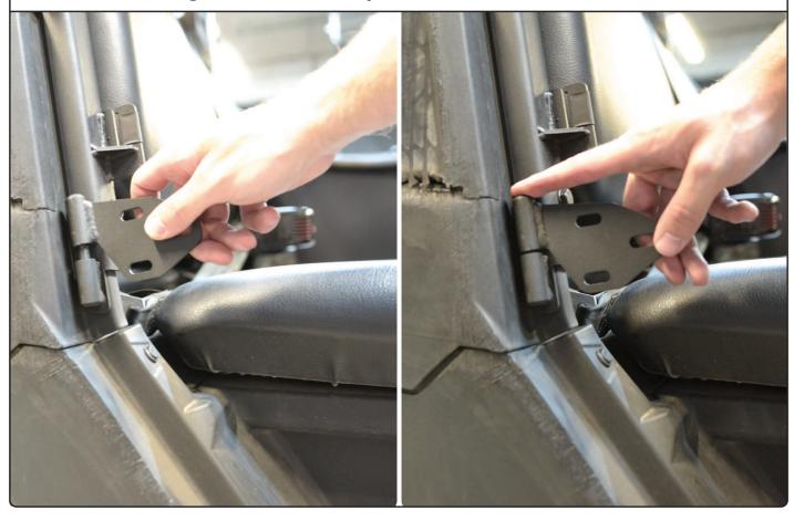
20. Install the bracket #9 in the upper door mount, install hinge D1, fix it with M6 bolts 1, washers 3 and 4. Do not completely tighten yet.
