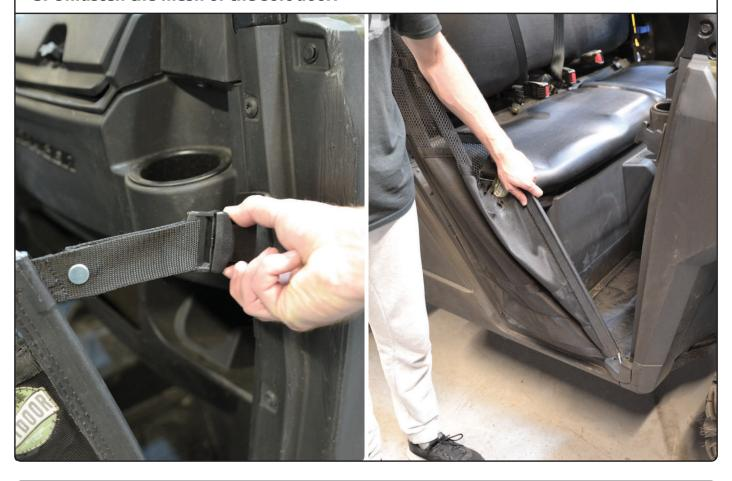
4. Unscrew the bottom bolt of the soft door, remove the soft door fixing and screw the bolt back.
