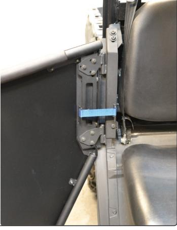
24. Close the door. Adjust door and brackets. Tighten all connections. Repeat for other side. REPEAT FOR OTHER SIDE.
