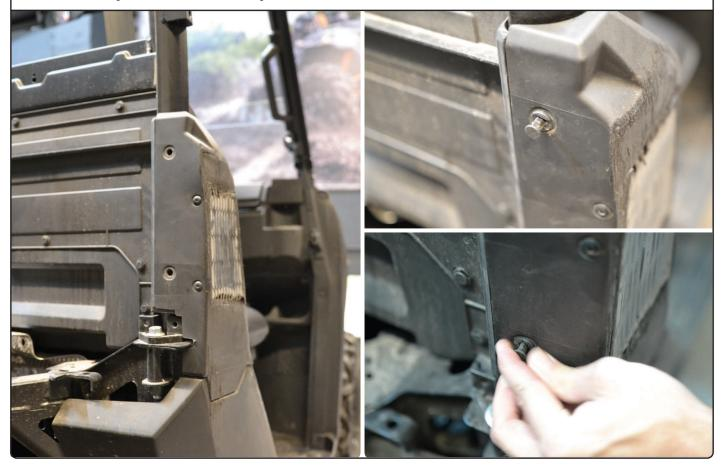
14. Install the bracket B2, in the upper part fix it with OE bolts, in the bottom fix it with M8 bolt 2, washer 5. Do not fully tighten the bolts.
