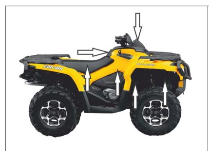
1. Remove plastic wing flaps from the both sides. Remove the seat, plastic sheet plate on the air filter, and plastic sheet plate on the dashboard. Plastic panels are at both sides of the seat. To dismount pistons, use of the special piston puller tool is recommended.
