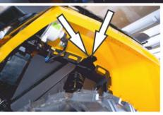
3. Remove the front luggage boot. Screw out the screws indicated with arrows from the both sides.
