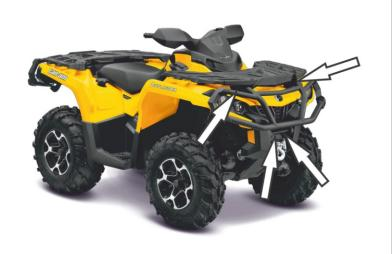
2. Remove the front bumper. Screw out 4 screws indicated with arrows. To make removing of lower screws convenient, remove the winch hawse pipe.
