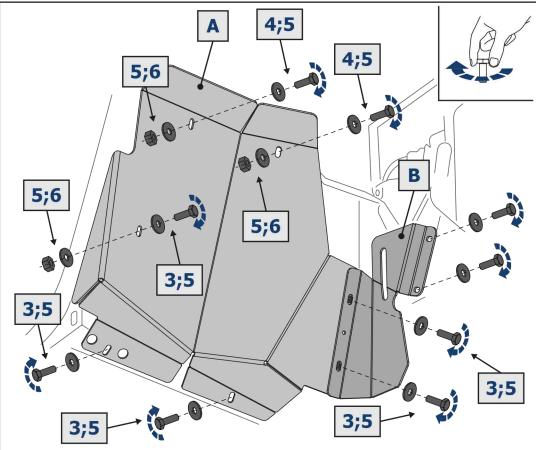
TIP: PERIODICALLY CHECK ALL HARDWARE AND RE-TIGHTEN IF NEEDED.
